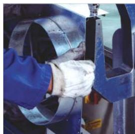
Optional process monitoring equipment ensures proper, consistent riveting with pedestal or automated systems.
